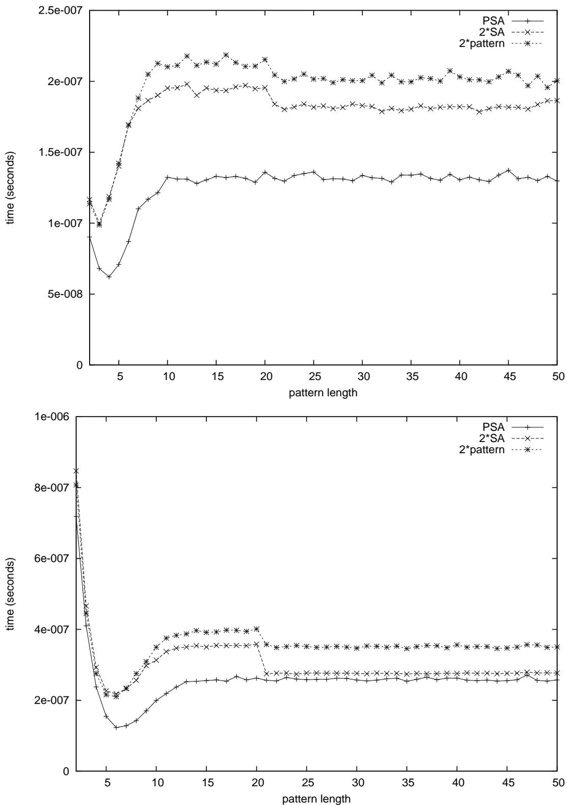
**Figure 2.** Comparison of running times for p-matching on random binary strings. The length of the text is 100 (upper) and 1000 (lower). The increase in time for short patterns is due to the increase of  $|P_{occ}|$ .
