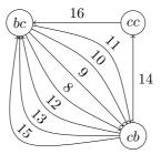
We are starting with the edge with label 1 and then we are traversing G along the smallest unused edges. If we end in a context with no outgoing unused edges, then we are continuing with the smallest unused edge. This gives the sequence (1, 2, 5, 3) after which we end in context aa with no unused edges available. Then we continue with the sequences (4, 6, 7) and (8, 12, 9, 13, 10, 14, 16, 11, 15). The complete sequence of edge labels obtained this way is
