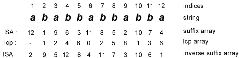
Figure 4. suffix array, inverse suffix array, and lcp array of ababbabbabba
