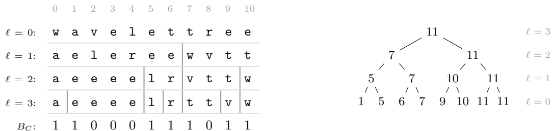
(a) The text re-ordering on each level and the bit vector B_C . The vertical lines mark the boundaries of the wavelet tree’s nodes.
