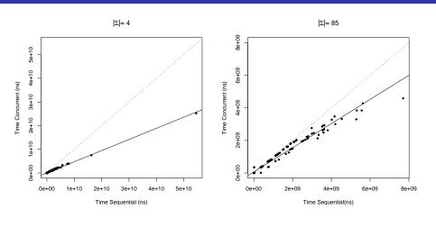
$$T_c = 39.6 \, \text{ms} + 0.47 \cdot T_s \qquad \text{for } |\Sigma| = 4$$
